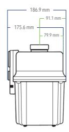
For pulse output version the recommended clearance required at the back of the meter for the output cable is 105 mm from the center line of the gas connections.
